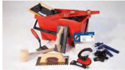
1- Installation of ceramic tiles should be carried out by skilled personnel, with demonstrable experience and appropriate tools and equipment, (i.e. toothed trowels, tile spacers, rubber mallets and suction cups for installation, and rubber trowels, sponges and containers for grouting). Check the information contained on the packaging beforehand, and meticulously follow the manufacturer's recommendations.
